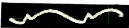
Fig. 12. Waveform at plate of horizontal output tube. This pattern is obtained when there is a shorted condenser between "B+" and boosted "B+" circuit.
