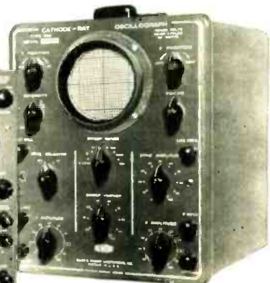
DuMont's Model 292—a 3" instrument for servicing.
