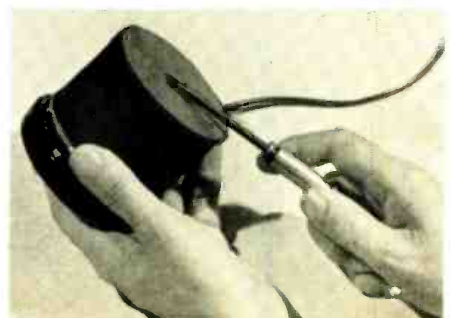
Fig. 6. How the demagnetizer can be used to magnetize service tools. A slight variation in operation permits this function.
