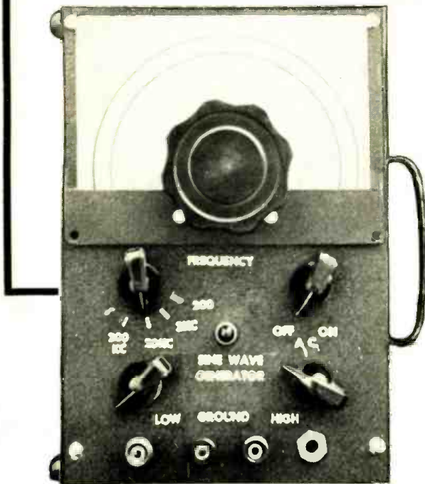
Fig. 1. Front cabinet view of home-built audio oscillator. The dial scale on author's unit is nonlinear in the interest of simplicity but may be made linear.
