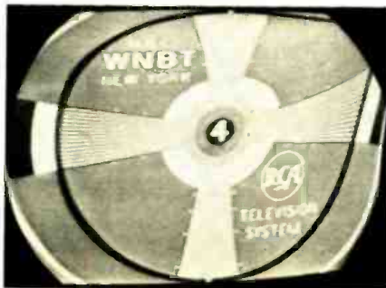
Fig. 5. Effect of magnetization on television pattern. Picture is distorted in the tube area which has been magnetized.
