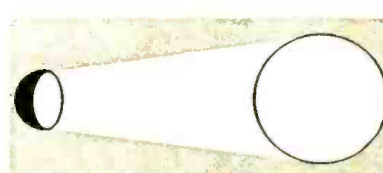
Fig. 5. The radiation beam of a parabolic reflector is circular as shown.
