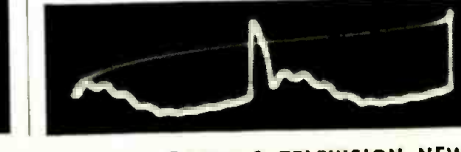
Fig. 14. Waveform at plate of horizontal output tube. Condenser shorted and series resistor across half of horizontal yoke winding subsequently was burned.
