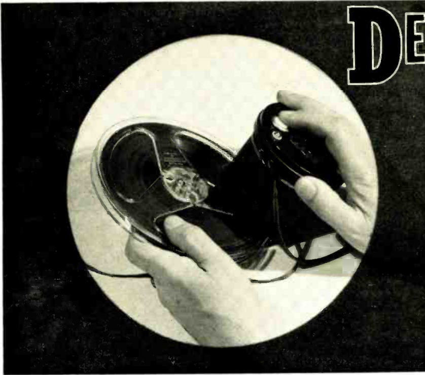
Fig. 1. Plastic reels of recorded tape can be demagnetized in a single operation by using unit described in this article.
